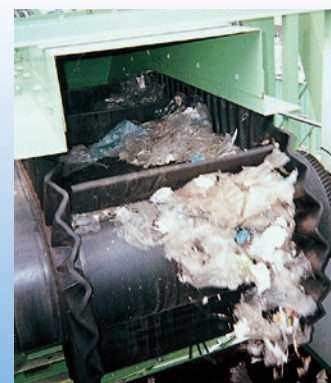
Waste plastic conveying
